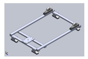
Assemble leveling system subassembly (p/n-LSA1) per assembly procedure
